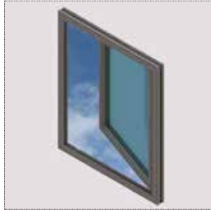
Side hung window outward opening
